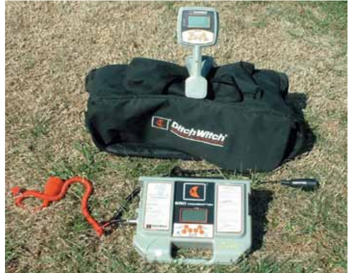
For toning, CommScope recommends equipment such as the DitchWitch 950R/T (shown above).
