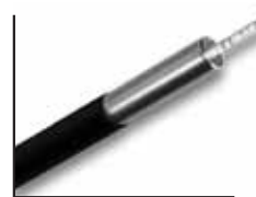
Residual dielectric and bonding compound on conductor after coring
