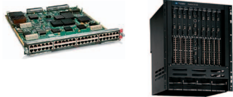
Figure 3.2 A high density switch module or chassis
